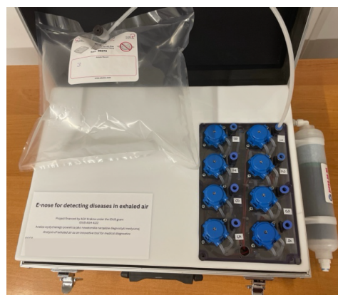
Figure 4. E-nose system used during measurements.
