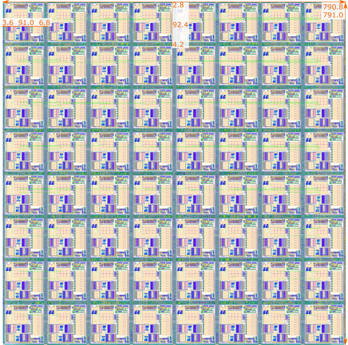
Figure 3.21: Layout of a single 8 \times 8 pixel group. Analog blocks and digital logic are separated spatially, and a central interconnect region contains shared resources, including transmission gates and logic.
