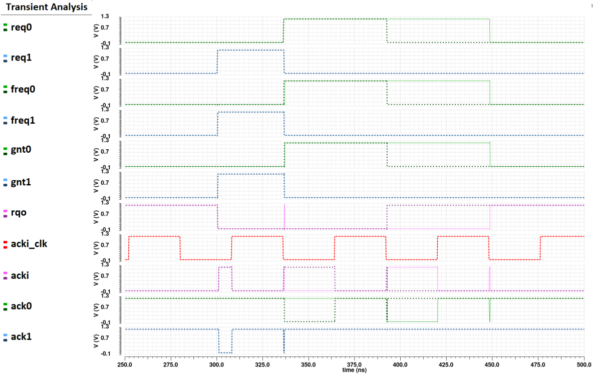
Figure 3.9: Waveforms from a tree composed entirely of Type II arbitration cells. The diagram illustrates cell behavior when multiple channels request readout, and a second request arrives either just before (dotted) or just after (solid) the acknowledge token.
