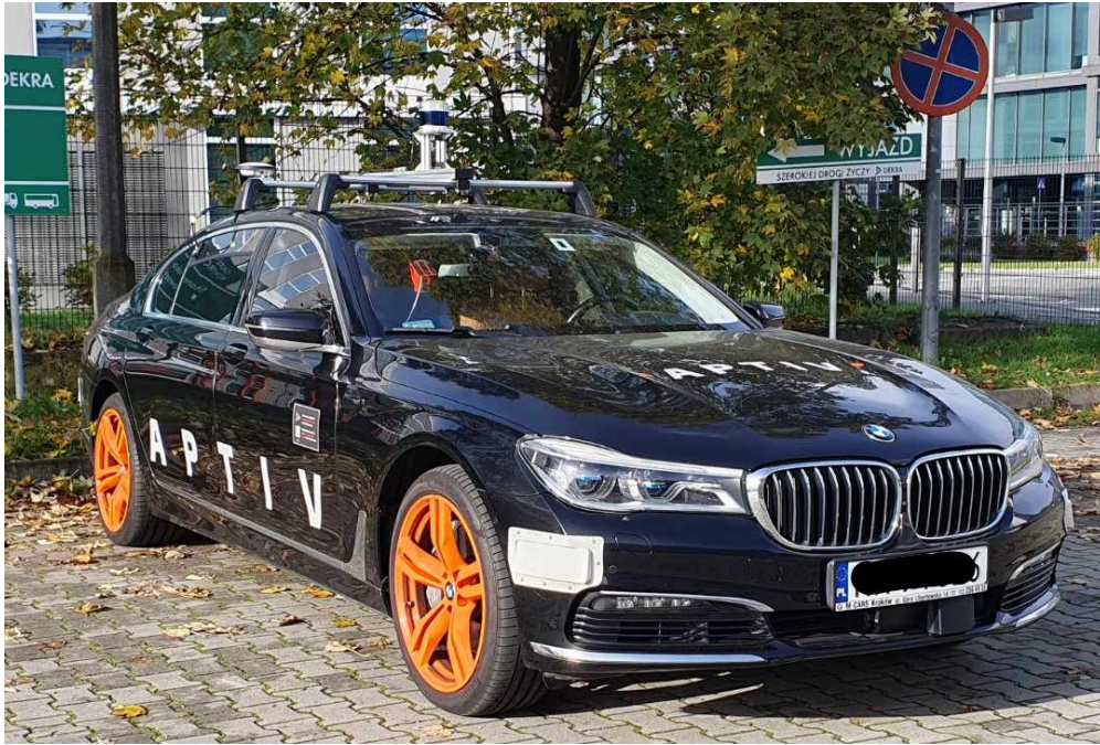
Figure 4.15: Aptiv test vehicle where RL-based parking spot planner has been integrated.
