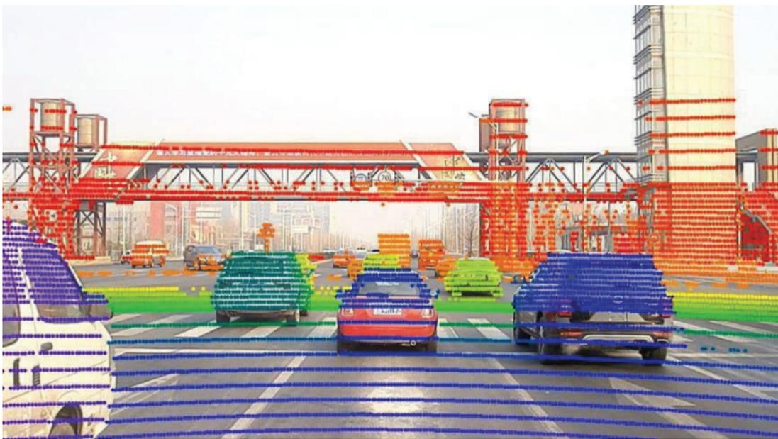
**Figure 2.3.** Pandora lidar measurements cast on camera image, color encodes distance. Source: Pandora lidar user manual, available at: <https://www.symphotony.com/wp-content/uploads/20181015-Pandora-Users-Manual.pdf>
