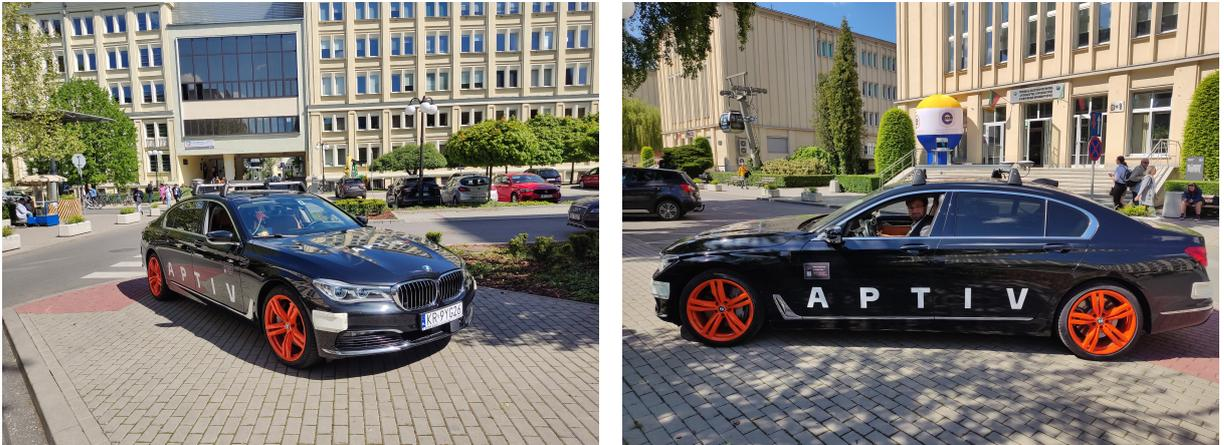
**Figure 6.1.** Pictures of the car. Lidar is mounted on top and radar is mounted on the grille, facing forward.
