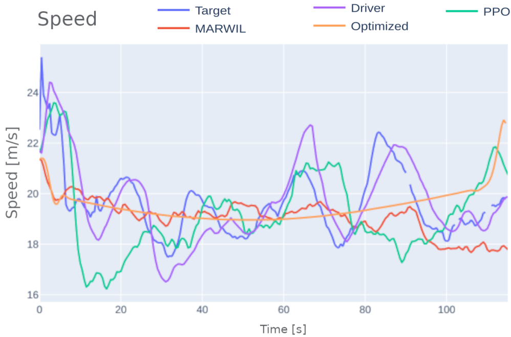
Figure 5.15: Comparison of executed velocity between different policies evaluated on resimulated log and the human driver.
