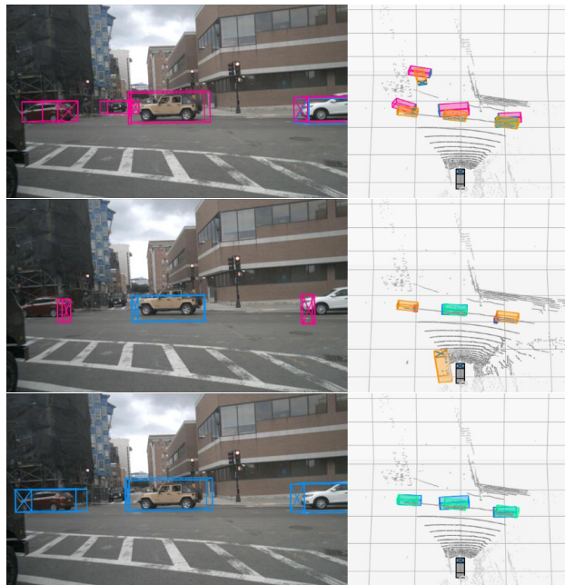
Figure 4.6: The comparison of the results for the same scene in the NuScenes test dataset, showcasing the outputs of the camera-only, radar-only, and CDSM fusion models from top to bottom. The presented image highlights the performance gain achieved through the fusion approach when compared to the single-sensor models.
