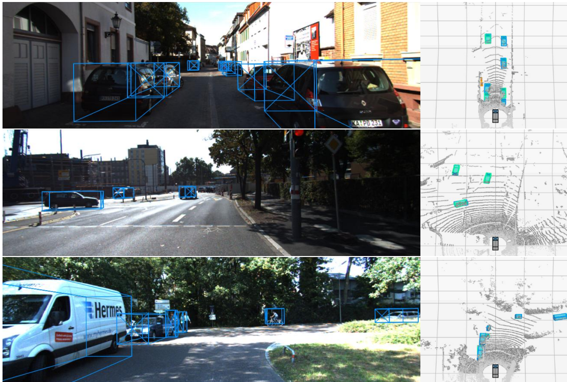
Figure 8.2: The results of CDSM fusion 3D OD model on KITTI test set. The visualization overlay employs a colour coding scheme that was introduced earlier, where labels are marked in green and predictions in blue.
