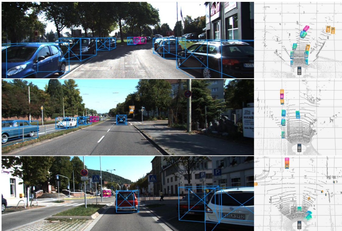
Figure 7.6: The results of monocular camera-only 3D OD model on KITTI test set. The visualization overlay follows a previously introduced colour coding scheme, with labels, positive detections, false detections, and missed ones marked in green, blue, magenta and yellow respectively. The pointcloud data is added for enhanced BEV visualization, however, it was not used for obtaining the 3D predictions, which are based on camera image alone.
