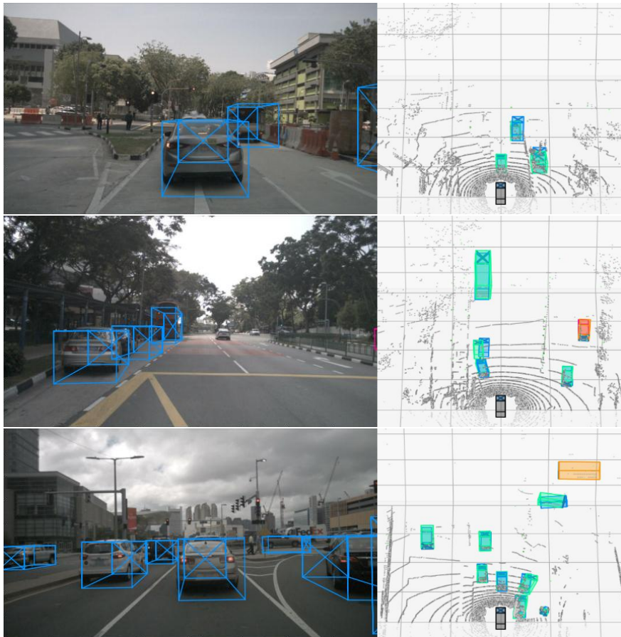
Figure 8.3: The results of CDSM fusion 3D OD model on NuScenes test set. The visualization overlay follows the previously introduced colour coding scheme: labels, positive detections, false detections, and missed ones are marked in green, blue, magenta and yellow respectively.
