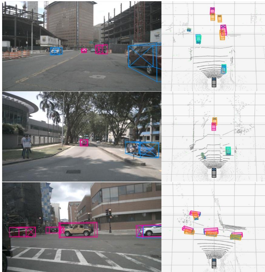
Figure 7.7: The results of monocular camera-only 3D OD model on NuScenes test set. The visualization overlay follows a previously introduced colour coding scheme: labels, positive detections, false detections, and missed ones are marked in green, blue, magenta and yellow respectively. The pointcloud data is added for enhanced BEV visualization, however, it was not used for obtaining the 3D predictions, which are based only on camera image.
