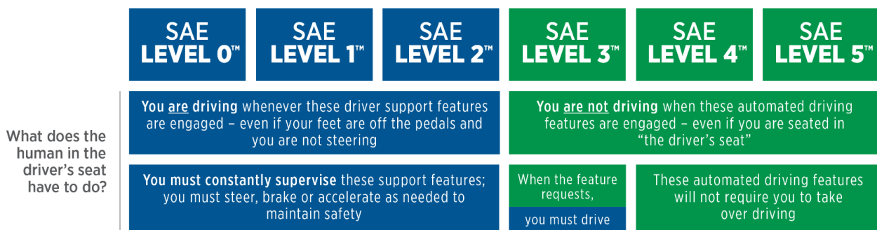
Figure 2.1: Classification of automation levels in AVs according to SAE. There are 6 distinct levels, from no automation to fully autonomous driving level. Source (Automotive Engineers 2018).
