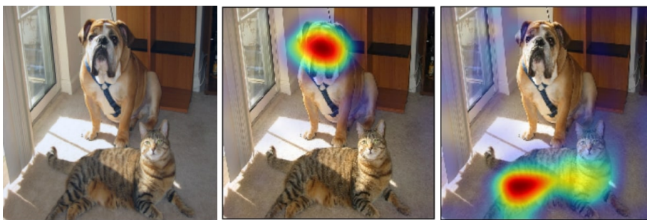
Figure 4.4: Results of Grad-CAM application for a classification network. The original image as well as CAMs for the "dog" and "cat" classes are presented from left to right. The results show that a dog is detected based on mouth features, whereas a cat depends more on fur patterns. Source (Selvaraju et al. 2017).
