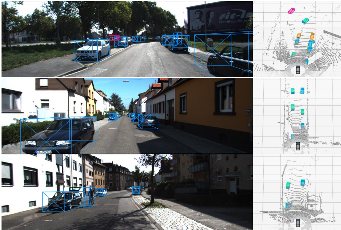
Figure 7.3: The results of LiDAR-only 3D OD model on KITTI test set. The visualization consists of two distinct views for each sample, namely the camera image and the BEV perspective. In the former, blue and magenta bounding boxes represent model predictions and false positives respectively. In the latter BEV, supplemental target labels are marked in green and missed detections in yellow. The LiDAR pointcloud data overlay is present in BEV but bypassed in the camera image for better overall visibility.
