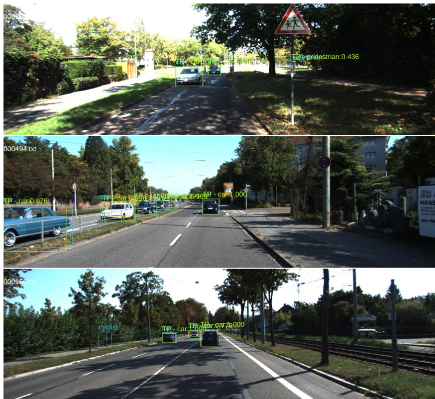
Figure 7.1: The results of camera-only 2D OD model on KITTI dataset test image samples. Blue bounding boxes represent dataset labels and yellow ones are model predictions. Both bounding box types have class name indicators above, along with confidence scores for the model predictions. "TP" denotes True Positive relationship between prediction and label according to the association method employed.
