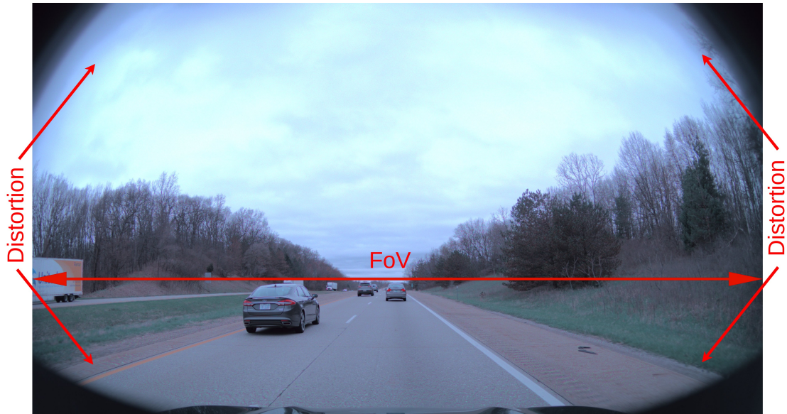
Figure 2.4: A sample from the automotive-grade camera. The key aspects of the presented image are wide FoV, which enables the capturing of more information from a single frame, and strong distortion, visible especially in the corners of the image. Sample from the industrial partner company demo car test drive.
