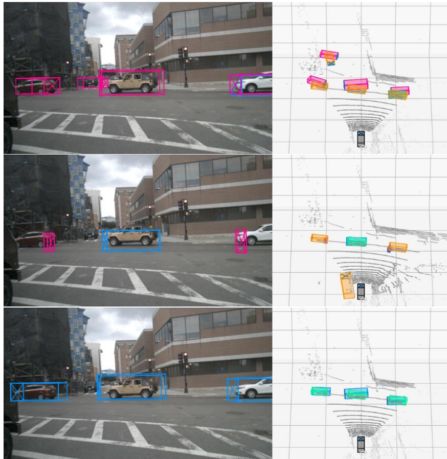
Figure 8.5: The comparison of the results for the same scene in the NuScenes test dataset, showcasing the outputs of the camera-only, radar-only, and CDSM fusion models from top to bottom. Both the images and corresponding 3D views are provided, along with a visualization overlay that follows the established colour scheme. In this colour scheme, labels are shown in green, positive detections in blue, false detections in magenta, and missed detections in yellow. The BEV also includes a LiDAR point cloud for reference. The presented image highlights the performance gain achieved through the fusion approach when compared to the single-sensor models.
