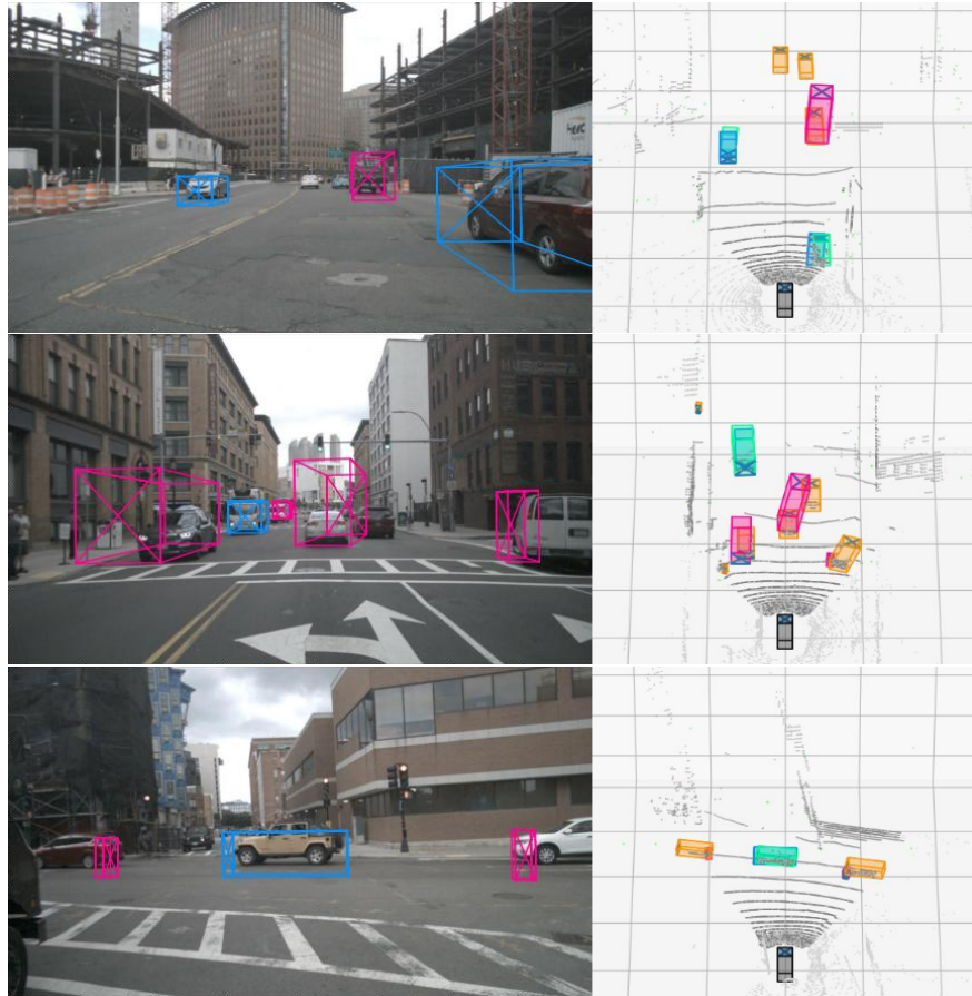
Figure 7.5: The results of Radar-only 3D OD model on NuScenes test set. The visualization overlay follows the same scheme, with labels, positive detections, false detections, and missed ones marked in green, blue, magenta and yellow respectively. Compared to previous experiments, Radar-only model provides significantly lower visual 3D OD results.
