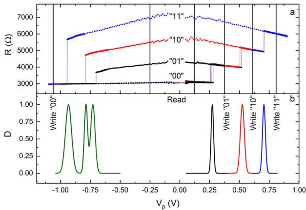
**FIG. 6.** (a) CIMS measurement of the two-bit memory cell. The proposed binary coding is also presented. (b) Switching voltages distribution, with regions for writing, and safe readout presented.
