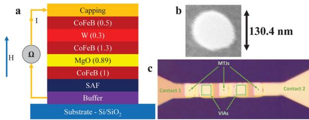
**FIG. 3.** (a) pMTJ layer structure, “SAF” denotes synthetic antiferromagnet,  $H$  denotes external magnetic field direction,  $I$  denotes current direction,  $\Omega$  denotes the sourcemeter or the cell driving circuit. (b) Scanning electron microscope image of a single pMTJ. (c) Micrograph of three serially connected pMTJs.
