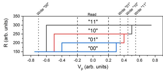
**FIG. 2.** Theoretically predicted resistance vs voltage applied to the proposed two-bit cell. Possible mapping between resistance and binary value as well as proposed voltages to write and read the cell is presented on the plot. Different colors represent the behavior of the cell after different writing voltages application.
