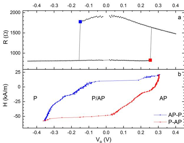
**FIG. 4.** (a) Representative  $R$ - $V$  loop of a single pMTJ, with switching voltages from P to AP (red) and from AP to P (blue) marked using big squares, measured without external magnetic field. (b) A stability diagram with marked regions where P, AP, or both of the states are stable.
