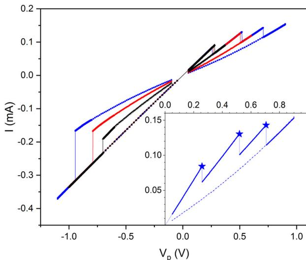
**FIG. 7.** Current changes during  $R$ - $V$  measurement for the storage cell constructed of three storage elements. Inset: a close up of current in the CIMS measurement for writing the “11” cycle. Critical currents causing subsequent elements to switch to the AP state are marked with stars.
