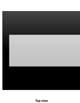
Figure 7.5: The UV photo-resist is exposed using UV direct-write process to transfer bottom electrode shape. After the exposure the sample is baked for 120 s at 95^\circ C
