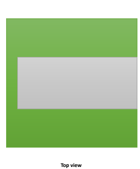
Figure 7.6: The UV photo-resist is developed using AR 300-475 developer bath for 20 s and then rinsed in deionized water ( DI-H_2O ) for 30 s.
