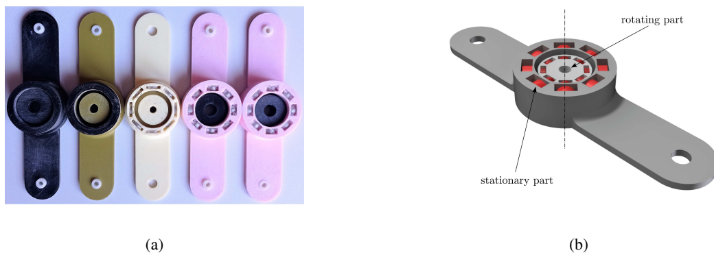
Fig. 9.12. Radial passive magnetic bearing prototype: (a) various 3D printed configurations, differing in the size of magnets and radial clearance; (b) an isometric illustrative model.
