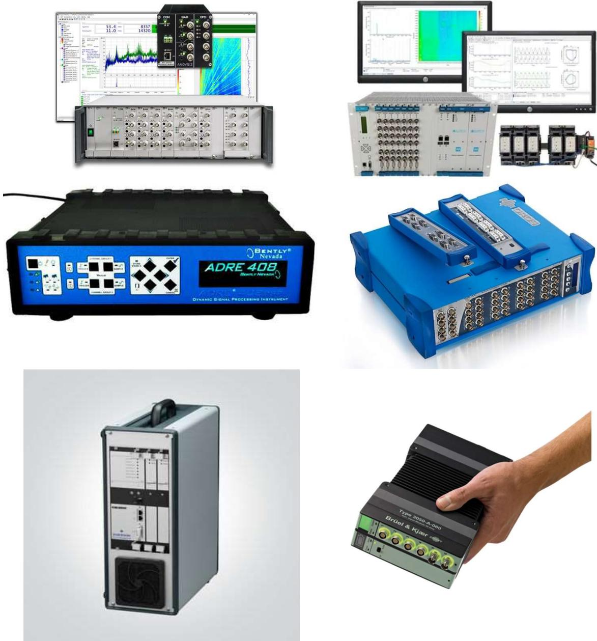
Figure 21. Examples of DAIUs from leading manufactures. The top: left – Siemens [18], right – Meggitt [19]; in the middle: left - Bently Nevada [20], right – OROS [21]; in the bottom: left – Emerson [22], right - Bruel and Kael [23].
