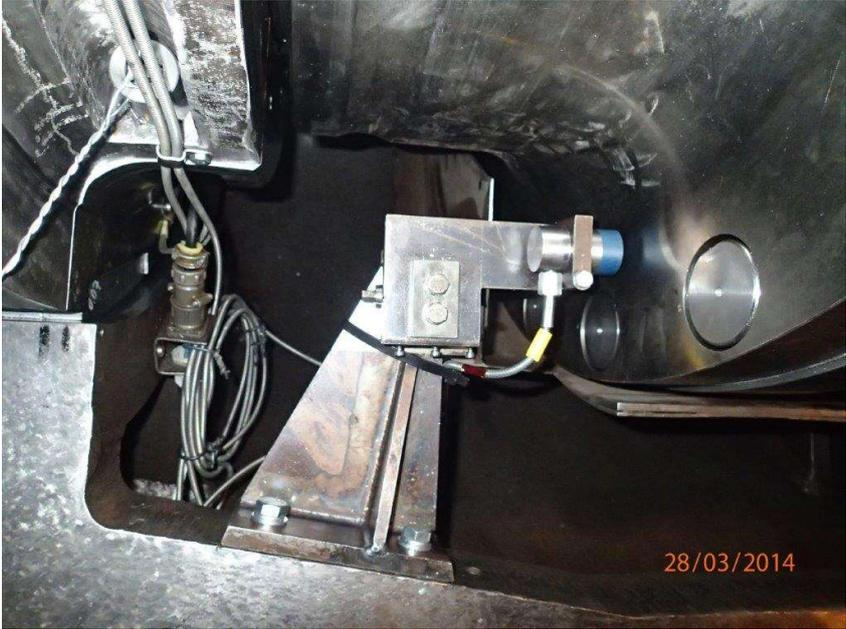
Figure 8. Relative expansion sensor assembly.
