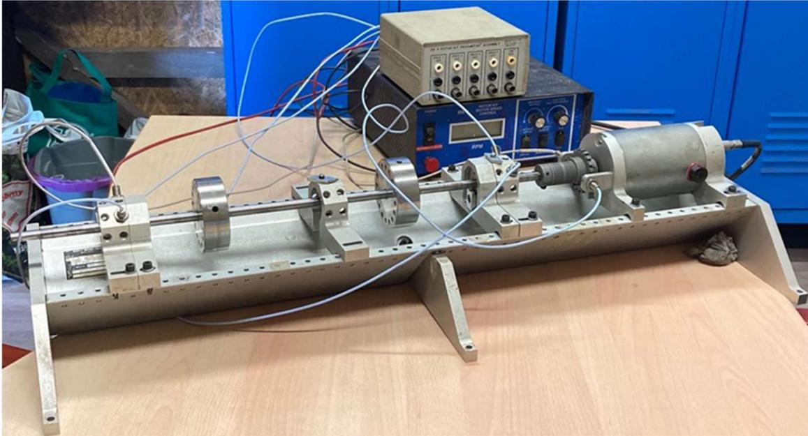
Figure 59. The Rotor Kit test rig used for model validation.
