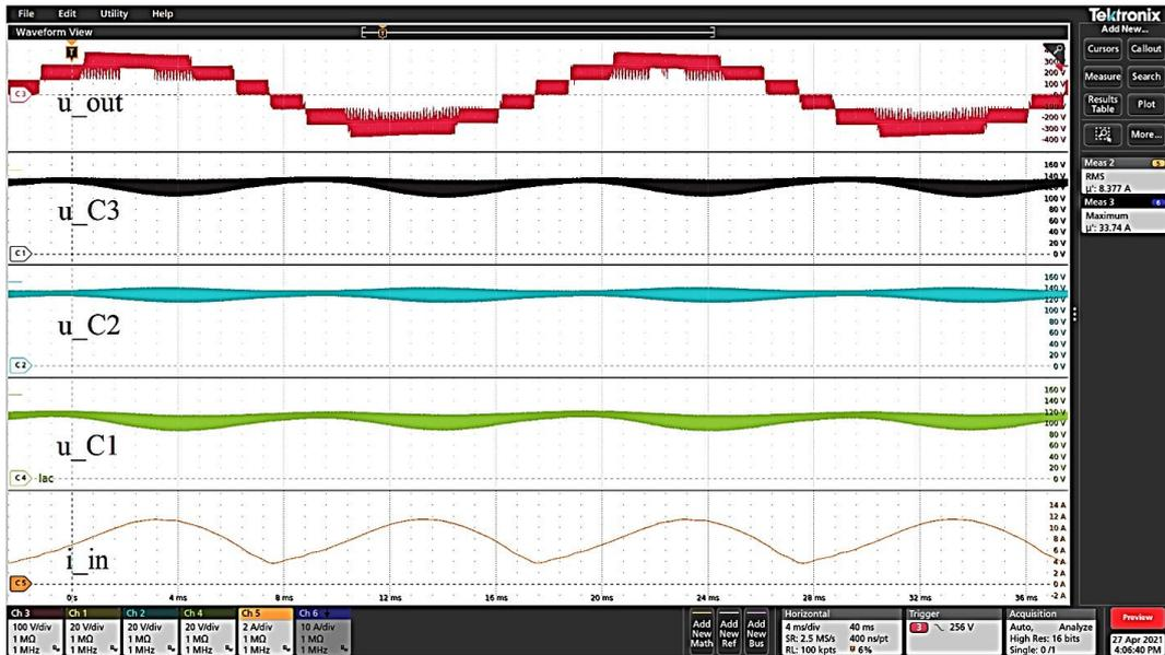
Figure 5.27: Operation of the balancer in the boosting mode for supplying the NPC inverter. The waveforms of the output voltage (100[V/div]), the voltage on the DC-link capacitors (100[V/div]) and the current of the DC power supply that was connected with the C2 capacitor (2[A/div]) [P.3].
