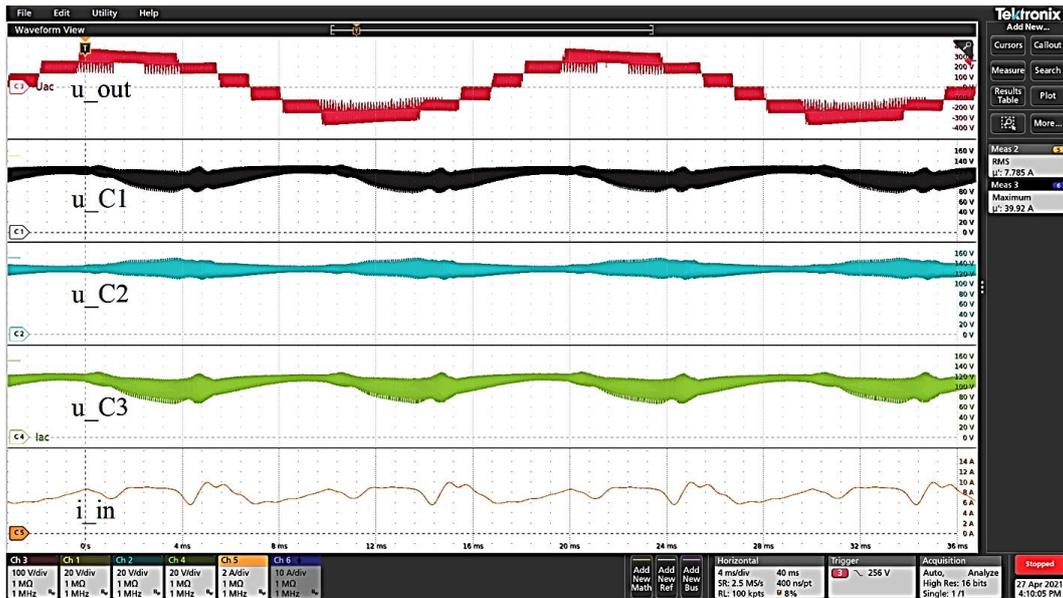
Figure 6.11: Operation of the balancer in the boosting mode and variable frequency for supplying the NPC inverter. The waveforms of the output voltage (100[V/div]), the voltage on the DC-link capacitors (100[V/div]) and the current of the DC power supply that was connected to the  $C_2$  capacitor (2[A/div]) [P.3].
