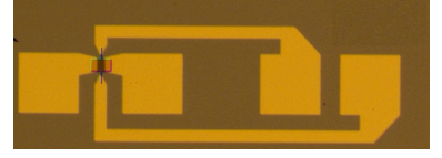
Figure 11: An example of the Hall bar planar device together with Ti/Au gold contact electrodes.
