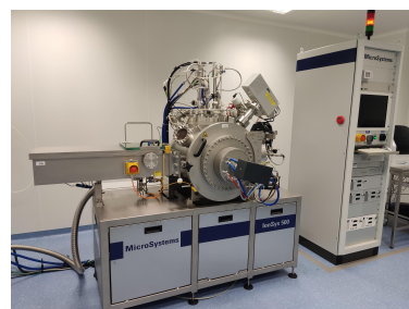
Figure 47: IonSYS 500 with integrated etching and magnetron sputtering system from Roth & Rau microsystems.
