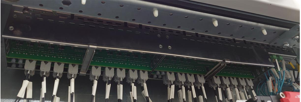
**Figure 5.7.** Control Hub with four Fiber Optic boards.  $4 \cdot 9 = 36$  cells connected.
