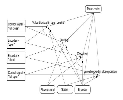
Figure 9.8: Causal graph for electromagnetic valve  $V_M$
