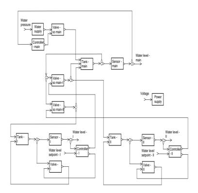
Figure 9.5: Schematic diagram of the tank system
