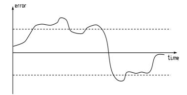
Figure 8.1: Simple example of error of a continuous observation and its upper and lower ranges
