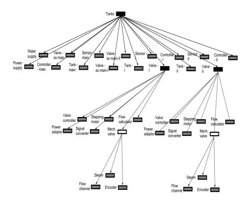
Figure 9.6: The tree of component structure for the tanks
