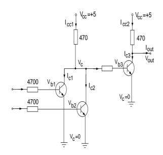
Figure 2.3: The OR gate realized by three npn transistors
