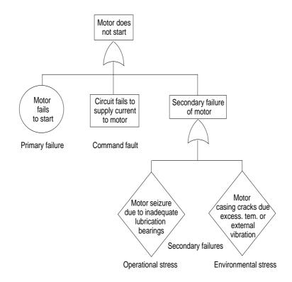
Figure 2.1: Example of a fault tree
