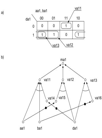
Figure 3.2: Graph AND/OR/NOT for an AND gate
