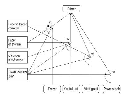
Figure 9.10: Diagnostic description for level 0 of hierarchical model of the printer
