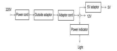
Figure 9.11: Diagnostic description for power adaptor
