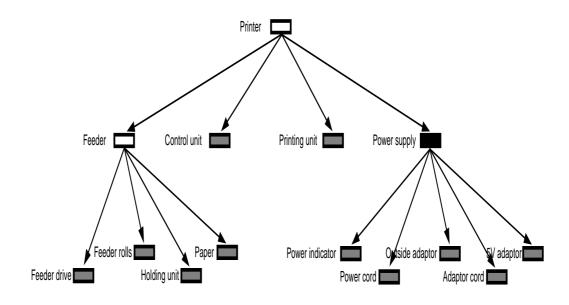
Figure 9.9: The tree of component structure for the printer
