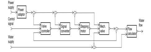
Figure 9.7: Valve schema
