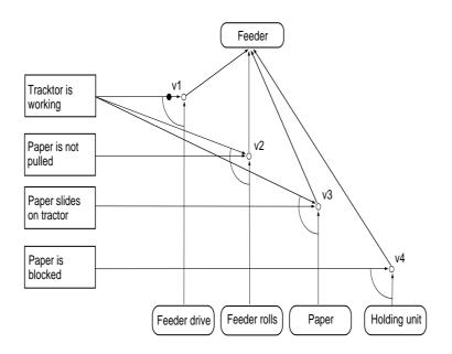
Figure 6.1: Diagnostic description for a printer feeder
