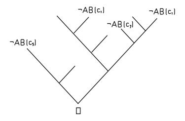
Figure A.3: Resolution style refutation tree for  $SD \cup OBS \cup \{\neg AB(c) \mid c \in COMPONENTS\}$  (figure for:  $\neg AB(c_1) \land \neg AB(c_5) \land \neg AB(c_7)$ )
