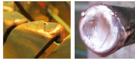
Figure 8. Left: Shape of the electrode fingers with a moving arc after test Right: Shape of cylindrical rod after a test with a stationary arc .
