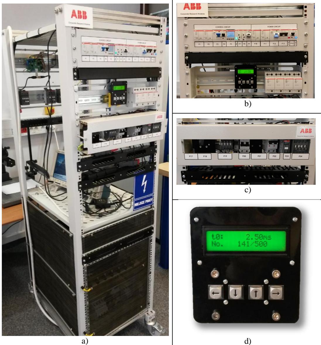
**Figure 6.18.** The laboratory stand: a) the overall view; b) the control panel; c) the panel with the operated switch (marked as P19); d) the LCD user interface with buttons
