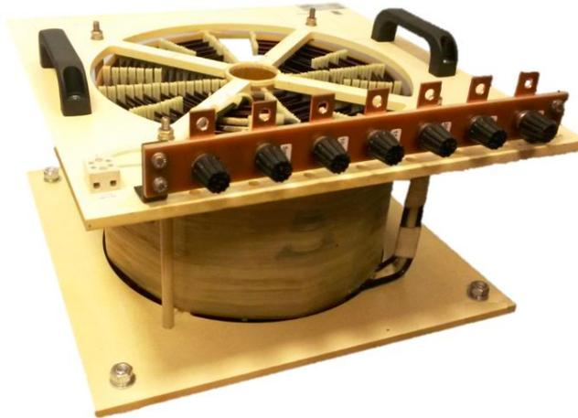
**Figure 6.19.** *The inductive air-core load used to perform the researches*
