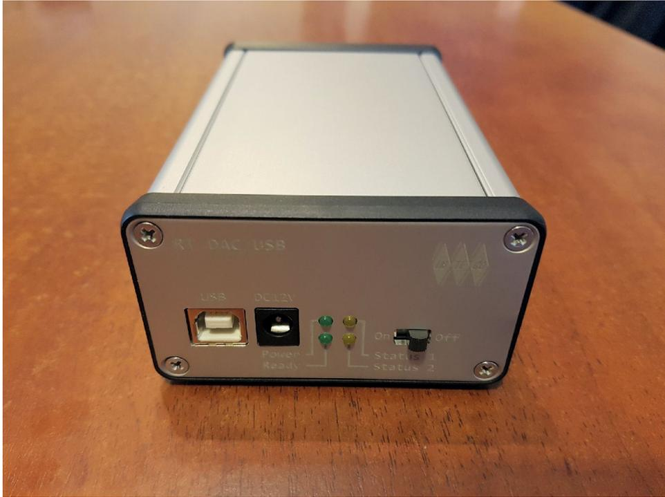
Figure 3.3: The picture of the RT-DAC/USB2 I/O board.
