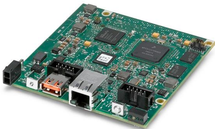
Rys. 6.9. Single-Board RIO firmy National Instruments (NI9606) [73].
